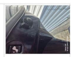
It works except I had to remove the washer from the Suzuki Flush M as the Tohatsu has an inbuilt washer.Voila it works. I will test it on the water (and carry the Tohatsu Plug in case) in the near future. Members with a similar flushing point may want to check them out as they have models for Mercury, Suzuki and Yamaha and Honda.
